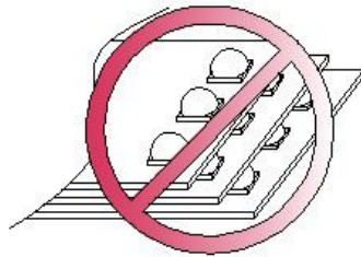
Do not stack assembled PCB
