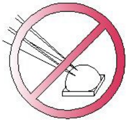
Do not poke the Led Lens with sharp object
